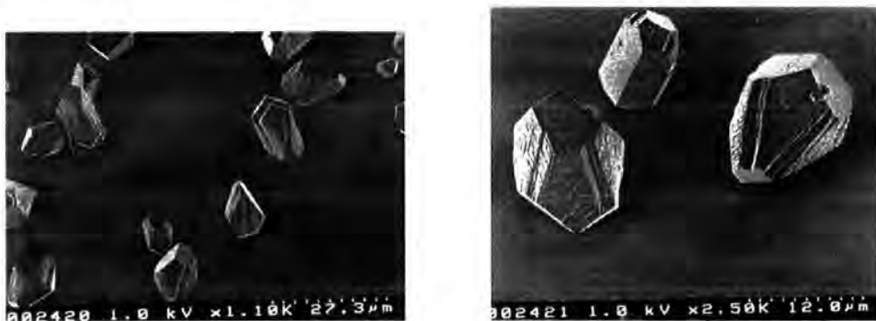
Fig. 3.3.17. Scanning electron micrographs showing \text{CaCO}_3 crystals grown from bulk solution in presence of model compound 4c [\text{Ca}^{2+}]:[\text{model compound 4c}] 100:1.
