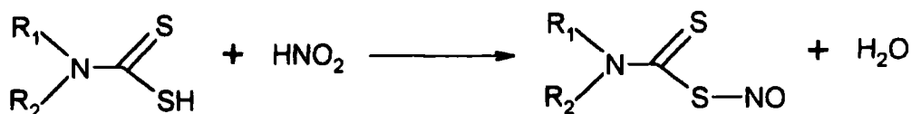
Scheme 5.3 Chemical equation for the reaction of nitrous acid with the dithiocarbamate functional group.
