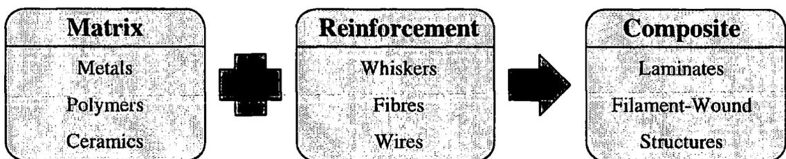
Figure A.1 Composite materials composed of matrices and reinforcements [2].
