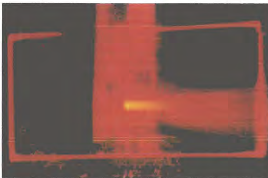
Fig.4.41 Beam branching effect in DCM waveguide film after irradiation for 30 mins.
