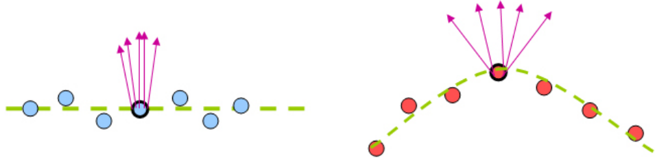
Figure 7.6: Visual representation of normal direction from bootstrap samples on a neighbourhood.
