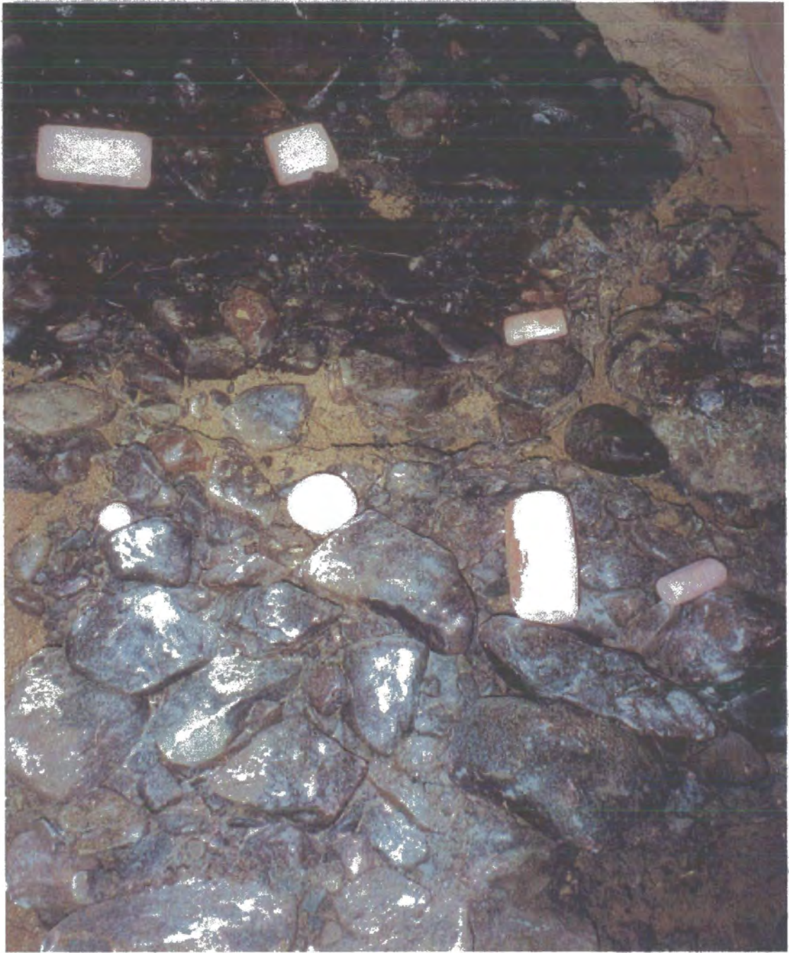
Figure 6.14 The undisturbed natural channel bed used to determine friction angles for particles of various shape, orientation, size and weight (Several of which are illustrated). Flow direction is from top to bottom of the picture. The field of view is approximately 65 cm across. From left to right axis of the large rod in the right of the photo is 96 mm.
