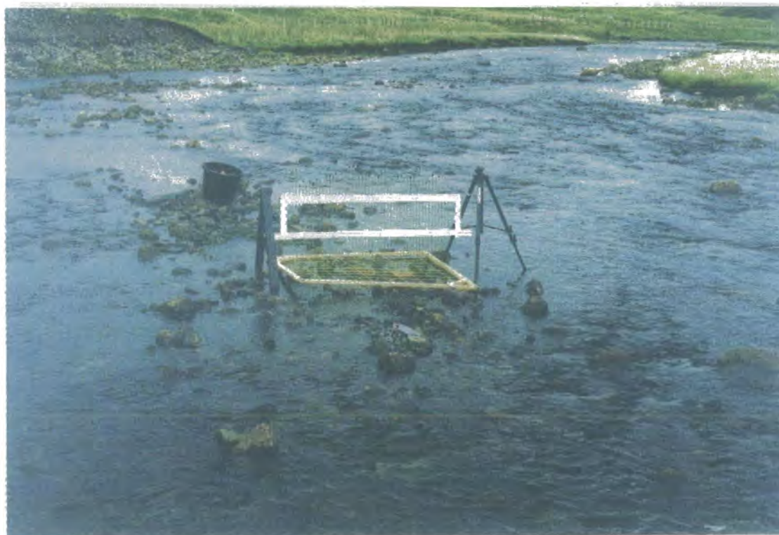
Figure 3.9 The pin (roughness) frame used to measure bed material roughness. The example shows the frame deployed at the Upper Tees site in a transverse orientation.
