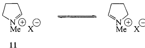
Scheme 4 Tautomerisation of the N-methylpyrrolinium salt (11) could explain the symmetrical incorporation of isotopically labelled precursors.
