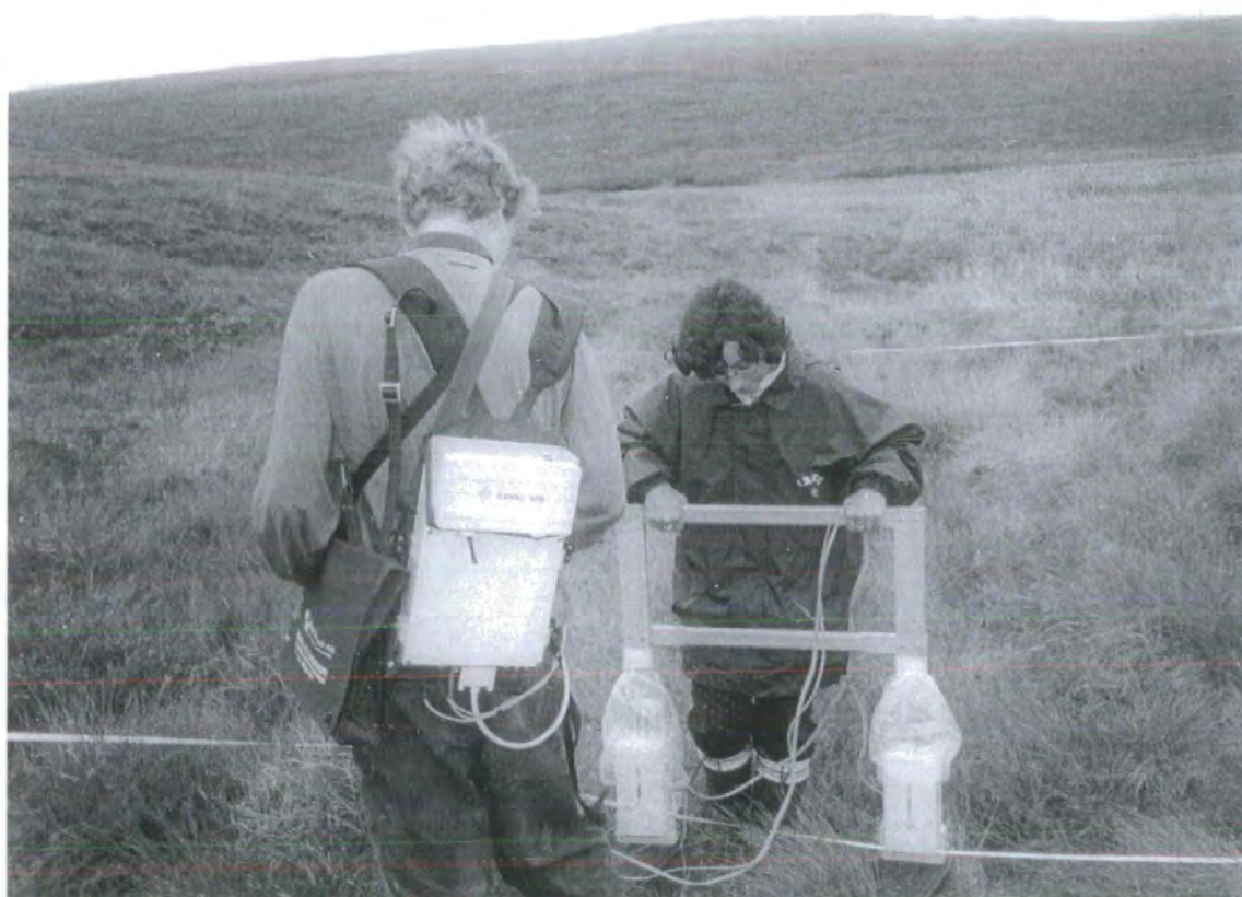
Figure 8.2. The best set-up of GPR equipment shared between two people for profiling long transects across peat. One person moves the antennae and receiver (fixed to a wooden brace) whilst the other carries the PC and control unit.
