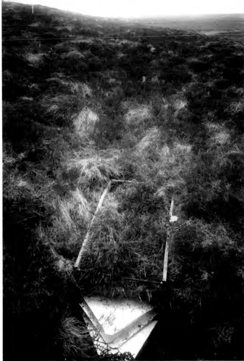
Figure 5.6. Observation of ponding development on runoff plots during rainfall simulation, a) ponding over almost the whole plot surface on bare peat, b) ponding in depressions on bare peat, c) bounded plot with runoff troughs on a densely vegetated peat surface illustrating the difficulty of witnessing ponding development on vegetated surfaces.
