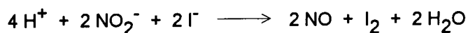
Scheme A3.2 H 2 SO 4 / KI / NaNO 2 calibration of the nitric oxide electrode
