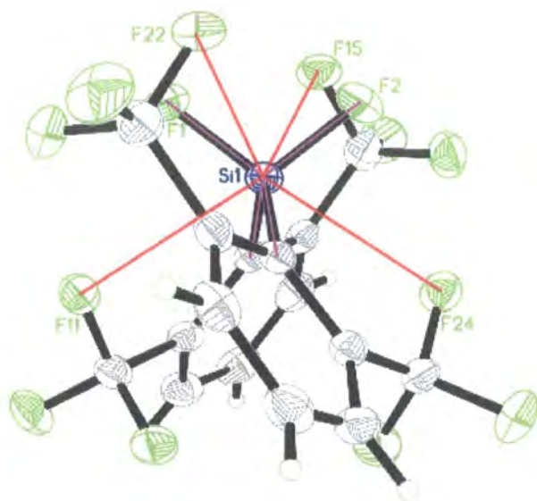
Figure 3.5: Si---F Short Contacts (covalent bonds are shown by a solid line and weaker interactions are designated by a red line)
