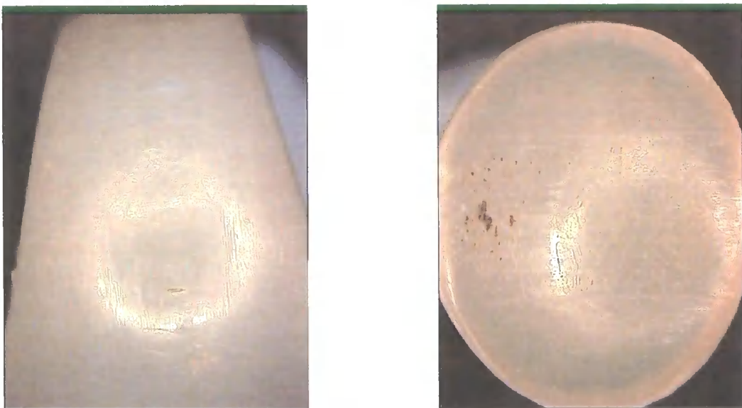
Fig. 7.2 Wear surfaces of the 8.5R non-irradiated XLPE prosthesis at the end of the test
