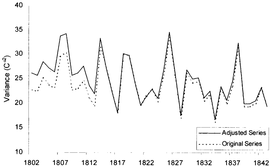
Figure 5.20 Adjusted (solid line) and unadjusted (broken line) temperature data reduced for Durham and adjusted to amend the variance to that of a series observed using just a single station, 1802-1843 (C 2 ).
