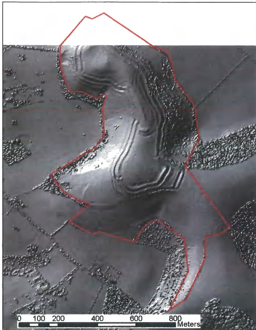
Figure 3.4: False shading image (produced with ArcGIS HILLSHADE command) of Hambledon Hill DEM. Red line shows boundary of NNR. The earthworks and areas of scrub, hedgerows and tree cover can be clearly seen.
