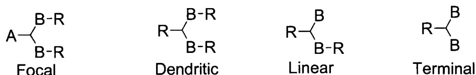
Figure 1.28 - The four types of sub-unit seen in the structure of a hyperbranched polymer.
