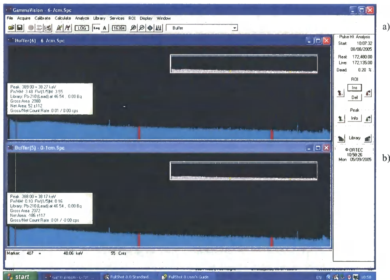
Figure 4.9: ^{210}\text{Pb} and ^{137}\text{Cs} results. a) MAIVK 6-7 cm; b) MAIVK 1-2 cm. The label on both the graphs indicates the position where ^{210}\text{Pb} is detected. If ^{210}\text{Pb} had been present
