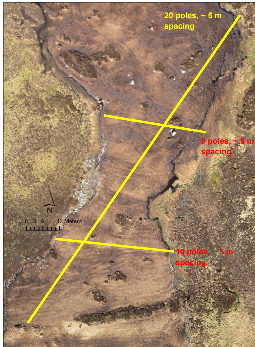
Figure 3.11: Yellow lines indicate the pole transects across the bare area of peat
