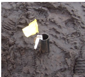
Figure 3.13: The Automatic Pressure Transducer installed in a well to measure the hydrological response of the blanket peat.
