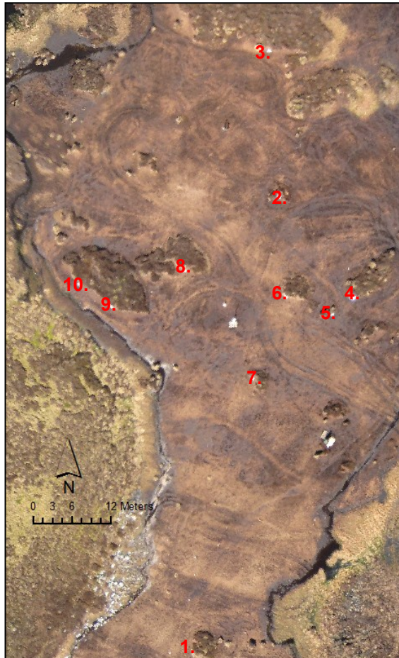
Figure 3.8: Location of Gerlach trough and erosion pin sites. The red numbers refers to the site number.
