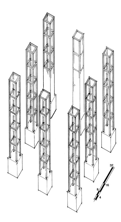
A movable system of platforms, stairs and walkways is deployed as the particular performance requires. All horizontal surfaces are wide enough for seating and access. The system provides connection between the towers, and can be used to cantilever into the volume of the cube.
