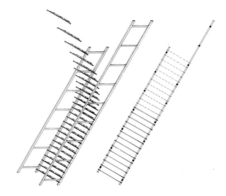
Floor planks (2 feet by 8 feet) provide a solid working surface. The interlocking pieces, attaching to both the joists and to themselves build the rigid stability of the floor.
