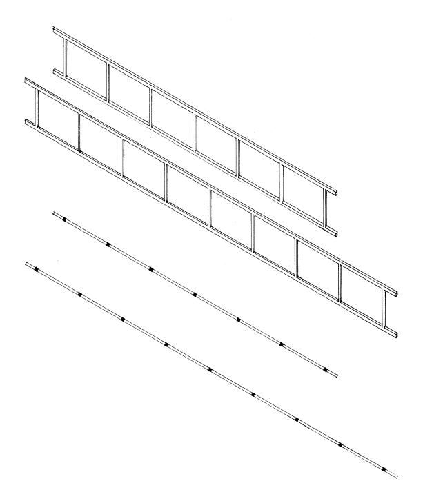
A set of lightweight floor joists are laid in between the trusses. These span the nineteen foot gap and begin to unify the structure.
