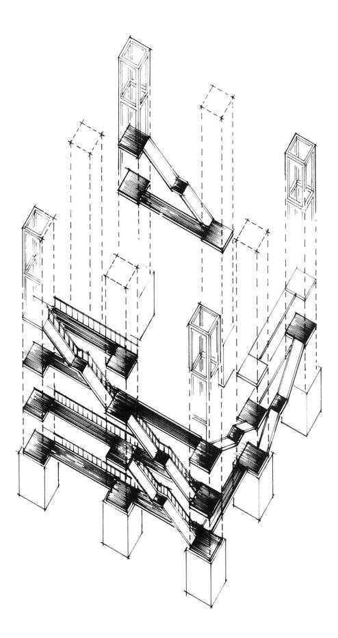
Two foot thick sound insulating panels are attached to the outside of the frame. These form a weatherproof surface, for some areas of the skin will be inside the building, and some out. A system of outer walkways provides circulation around and up and down the outside of the cube, for both performers and audience.
