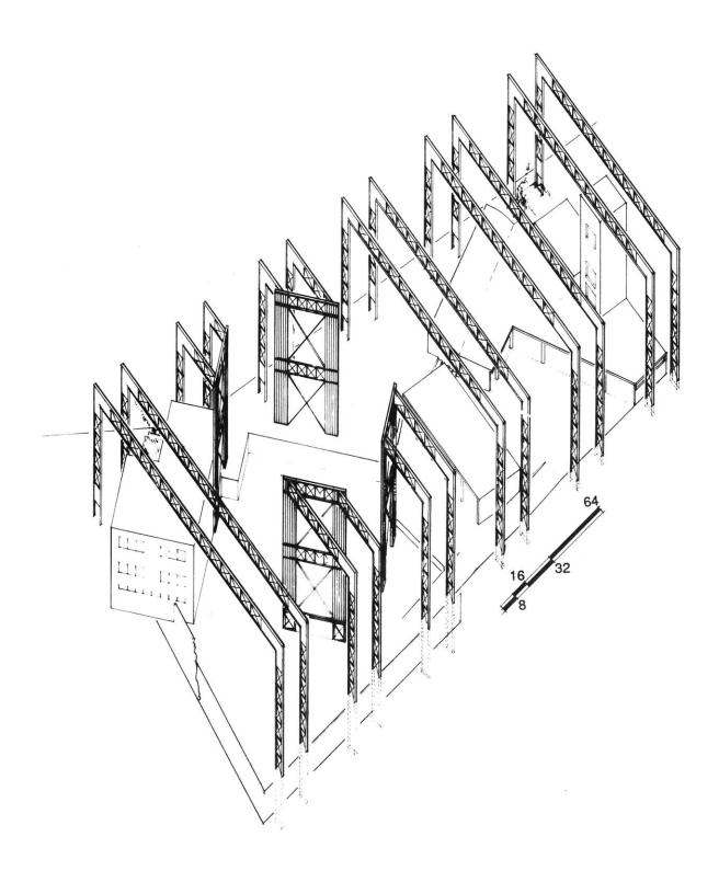
Here the cube and the four office elements are in place. The cube is planted firmly in the ground. The steel screens, parallel to the cube's surfaces, stay eight feet away. The four office and lab pieces are freely arranged, hanging from the structure. The longest piece extends into the zone of the cube, allowing easy connection to the performing space. Thus the last lab becomes a sound and control room for the cube.
