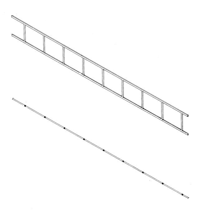
The framework for the labs and offices begins as two large Vierendeel trusses, perhaps of different lengths.
