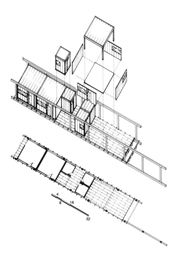
An access walkway is suspended from the outside of one of the Vierendeel trusses. This provides entry into the labs, the spaces between the offices, and to the lounge. The walkway can also continue, freely in the air, to intersect with other areas that lies beyond.
