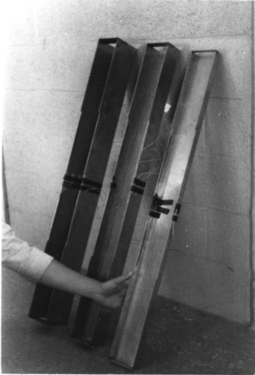
Figure 3: Photo - Channel Test Sections Showing Strain Gages
