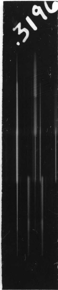
Figure 2-a. Photograph of Zeeman pattern showing no magnetic splitting. The line is 3196.591 (50,2) classified as  $a^5F_1 - g^5D_0$ . The p component is at the top, zero-field line in center and n component in the bottom exposure. Set number Z-49.
