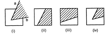
Figure 6.10: (i) The polygon corner defined by edges a and b. (ii) The pixel mask resulting from edge a. (iii) The pixel mask resulting from edge b. (iv) The result of "and"ing the two masks. This is the final pixel mask in the mask buffer.
