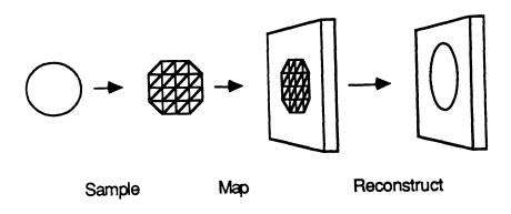
Figure 3.1: Sampling, mapping, and reconstructing a surface.
