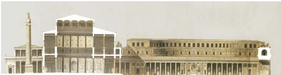
FIG. 109 Section through the axis that connects the Templum Pacis, through the forum of Trajan and the Basilica Ulpia, to the Trajan's column. Reconstruction drawing by Julien Guadet, 1867.
