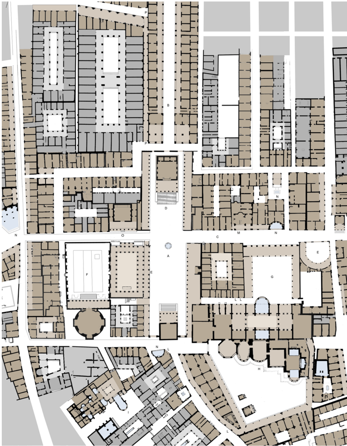
FIG. 87 Plan of Ostia, the harbor city of ancient Rome. A) Forum, the definitive layout is achieved during the reign of Hadrian (117-138 A.D.), B) Cardo Maximus is flanked by shops behind porticoes. C) Decumanus Maximus , D) Capitolium (120 A.D.), E) Basilica (81-117 A.D.), F) Round temple with forecourt (222-235 A.D.), G) Forum of the Heroic Statue (350 A.D.), H) Baths of the Forum (ca. 175 A.D.), I) Byzantine Baths (390-425 A.D.), L) Latrines , M) Basilica Hall (238-244 AD), N) Nymphaeum or fountains, O) Curia (81-117 AD), P) Via Tecta , one of the first covered streets (120 A.D.)
