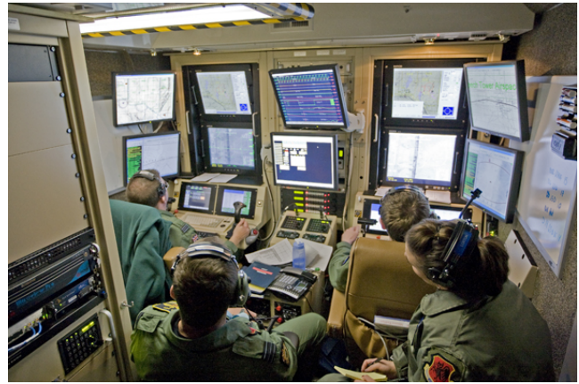
Figure 1: Cockpit control center for a Predator UAV. A pilot and several sensor experts collaboratively control the aircraft remotely, although their effort is split between different functions. The unofficial role of the observers is to ensure that the pilot has everything that he needs so that he doesn’t need to leave the controls. Image courtesy of Bryan William Jones.
