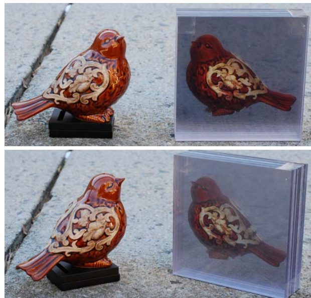
Figure 1: A real object next to a multilayer model fabricated in acrylic using our proposed algorithm.
