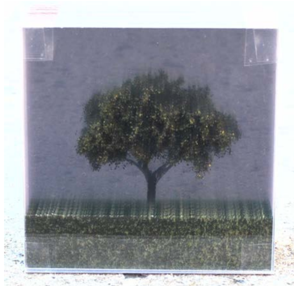
Figure 14: A 10-layer model of a tree constructed from polycarbonate and acetate sheets, viewed from approximately 20^\circ above the principal view direction. Objects with very thin features such as this tree cannot be printed using additive 3D printers.
