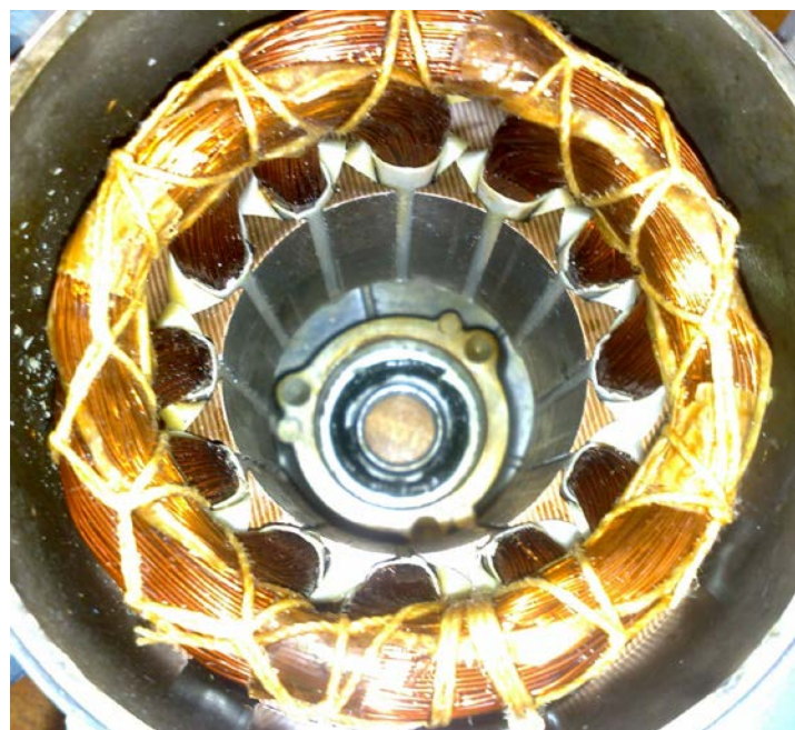
Fig. 5.1.2 The bundled and crossed over coils in a real motor
