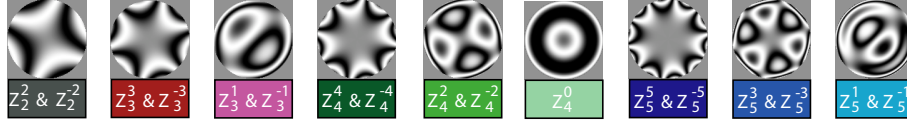
Fig. 2. Interferograms depicting the resultant zernike pairs using Eqs. 1 and 2. As the values of the Zernike coefficients C_m^{\pm n} in each pair change the amplitude and angle of the interferogram will vary. The colour code under each image will be used below in section 3. Z_4^0 has been included for completeness.
