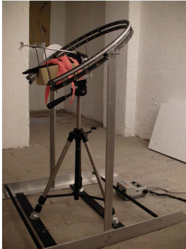
Figure 6-2. Photograph of the experimental apparatus used to measure visual fields in birds. The bird's body is restrained in a foam holder with its head secured by a bill holder custom-built to fit each species. The head is positioned so that the eyes lie at the centre of the sphere delineated by the rotating semi-circular arm. An ophthalmoscope is used to record the angle of limits of the bird's visual field, read off from the semi-circular arm. The arm is then rotated 10 degrees and the process is repeated.
