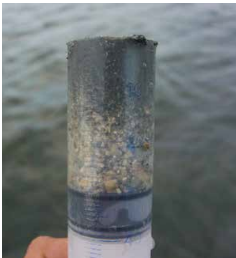
Figure D.2. Sediment corer used to quantify oxygen penetration depth. Consistently darker sediment indicates anoxic sediment, as indicated by a white arrow.
