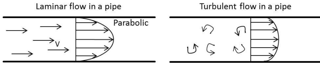
Figure 3-20: Effect of the turbulence in pipe flow with corresponding velocity profiles
