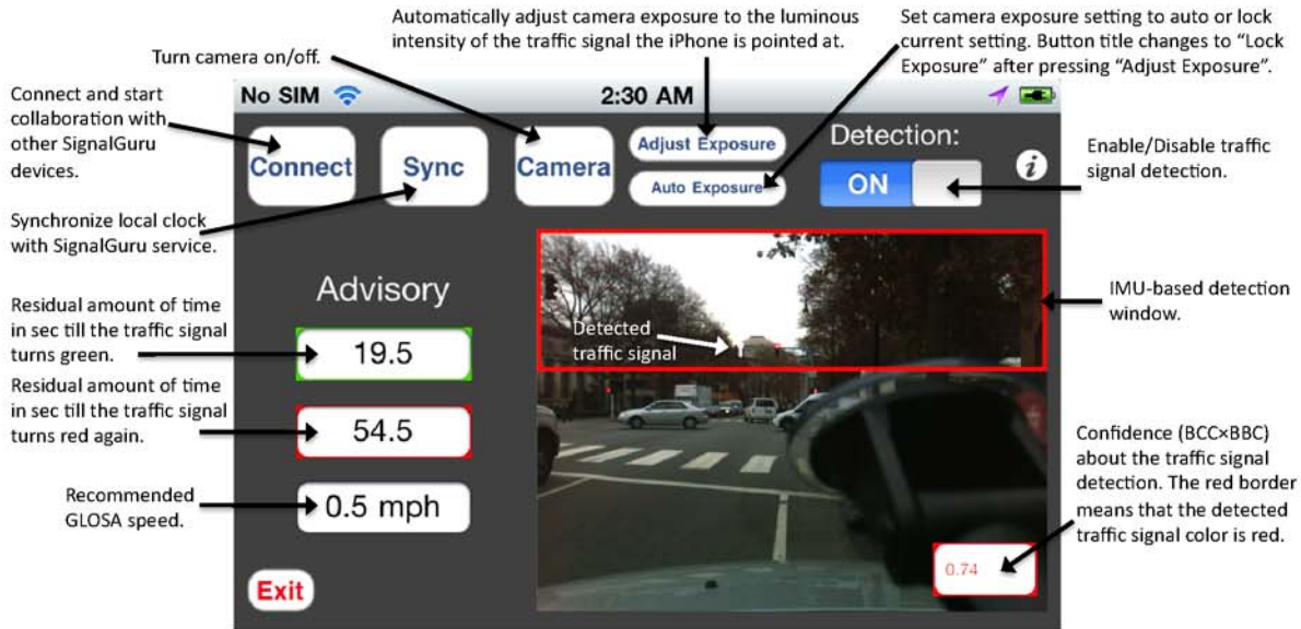
Figure 6: SignalGuru service screenshot. GLOSA advisory has also been included in the same iPhone application. Audio advisory can complement the visual advisory to alleviate driver distraction.
