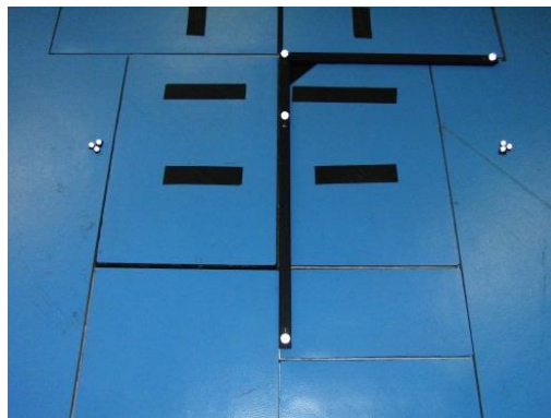
Figure 35. – Photograph of Kistler platforms, with the “L” shaped structure (LBMF, FMH).
