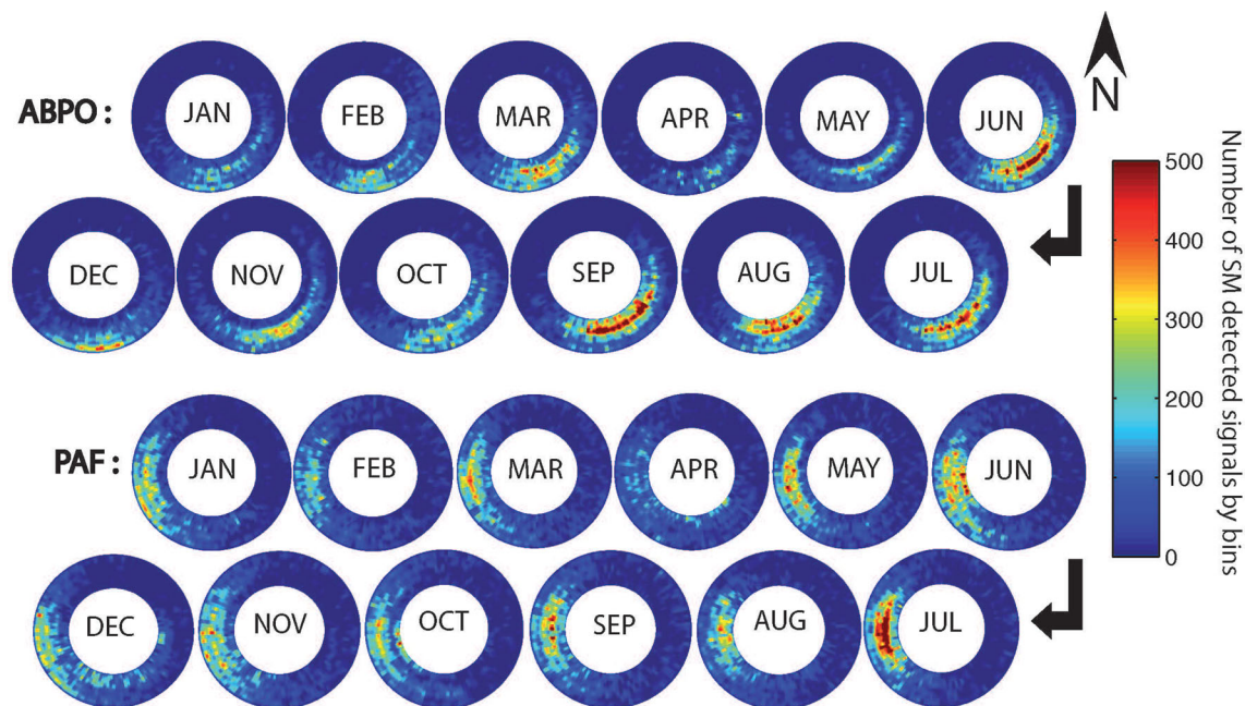
Figure 4. Monthly variations of SM polarized signals detected at stations ABPO and PAF throughout the year 2011. Every polarization diagram corresponds to one month of measurements where each detection is characterized by its backazimuth (indicated by the angle with respect to north) and its frequency (indicated by the radius). Inner and outer circles correspond to 0.09 and 0.17 Hz (around 6–11 s), which are the limits of the SM frequency band. The colour indicates the number of polarized signals detected by bin of 3^\circ for the backazimuth and of 0.01 Hz for the frequency. Red colours correspond to the maximum number of SM polarized signals detected by bins, which is saturated at 500.
