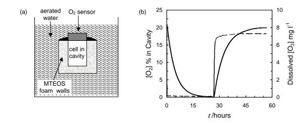
**Figure 2** Comparison of oxygen levels between a sealed system (lower curve) and one using the superhydrophobic foam (upper curve) to allow oxygen replenishment during consumption of oxygen at a rate 246  $\mu$ l h<sup>-1</sup> due to the discharge of a zinc-oxygen cell.
