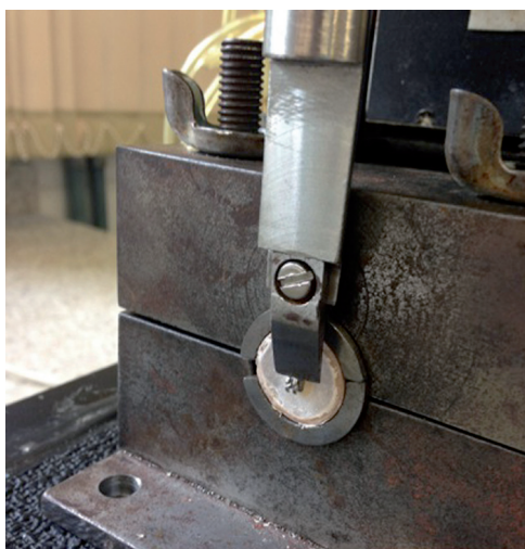
Fig. 3: Specimen adapted to a shear-testing device.
