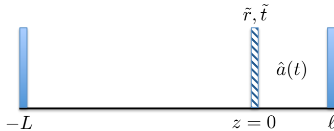
FIGURE 1.2: Open cavity bounded by a perfect mirror at z = \ell and a semitransparent mirror at z = 0 . The auxiliary cavity bounded by a perfect mirror at z = -L is for the quantization procedure.
