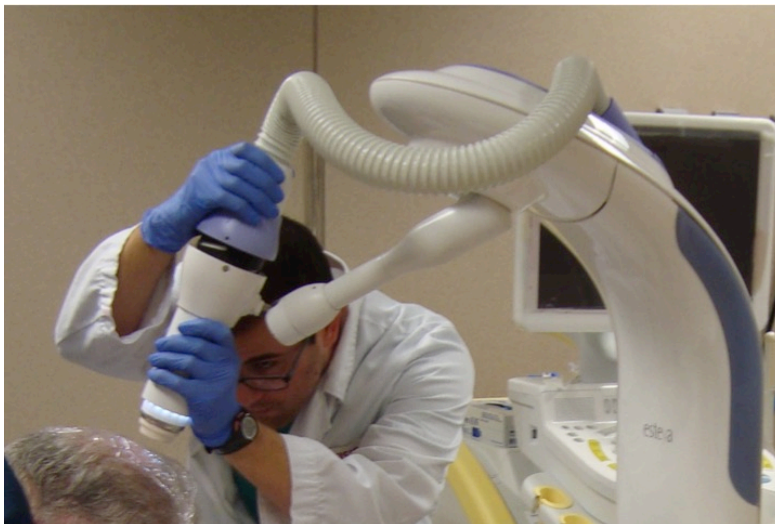
Fig. 2. The Esteya arm has several degrees of freedom in order to place the applicator.
