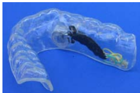
Fig. 1. Saliwell GenNarino electrostimulator containing the electronic system embedded in the plastic splint.
