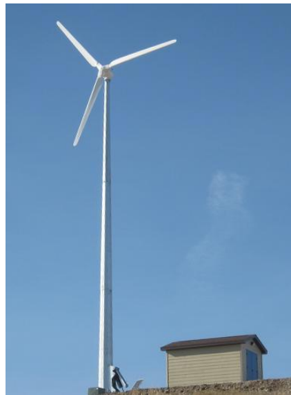
Figure 6. REDriven 3 KW wind turbine with three blades, Source: http://www.roanokecountyva.gov/DocumentCenter/Home/View/2018
