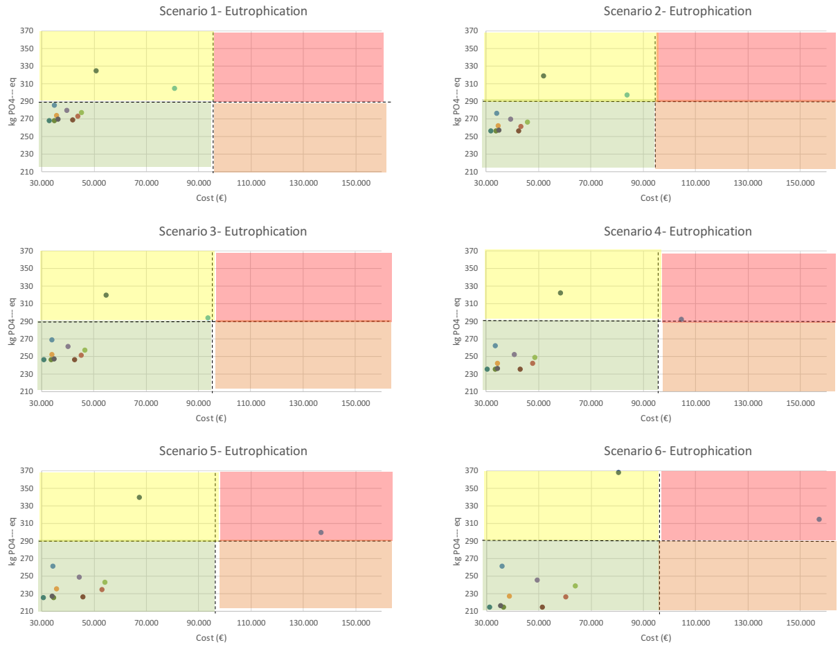
Figure A22. Eco-efficiency analysis: environmental impact (Eutrophication, kg PO4 eq) vs economic cost (€)
