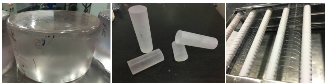
Figure 7.2: Relationship between the intermediate \text{Al}_2\text{O}_3 with different shapes and the total length of sapphire crystal rods
