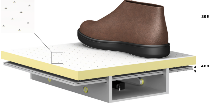
Figure 2: CAD view of 2D variable-friction floor tile using low-friction covering and sharp pins. The sole of the shoe is also covered with a low-friction film. The coefficient of friction would be controlled by varying the protuberance of the sharp pins.
