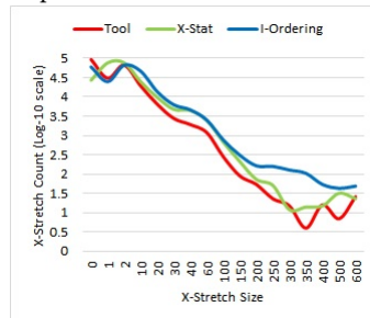
Fig. 8. Don't care stretch statistics for b19 circuit (Tool vs X-Stat[Trinadh et al 2014] vs I-Ordering)
