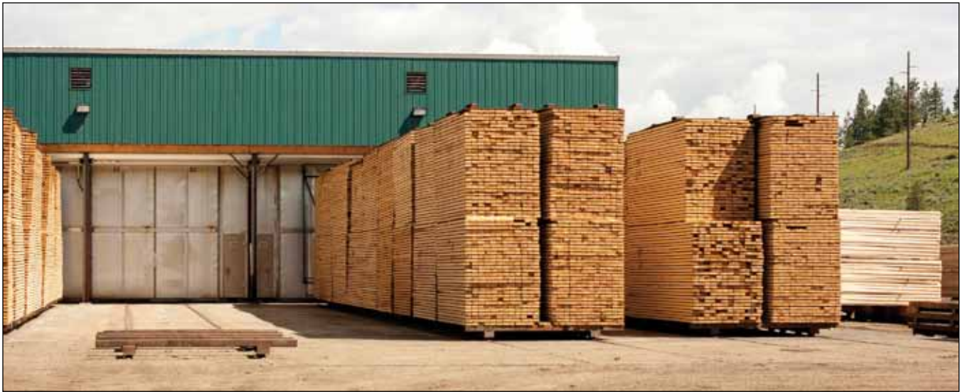
Figure 5-13—Dry lumber outside of kiln waiting to be restacked.
