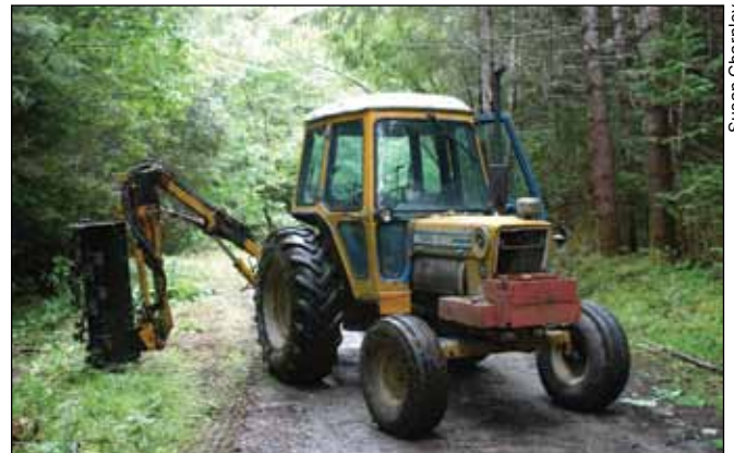
Figure 4-9—Machine used for mechanical brush removal.
