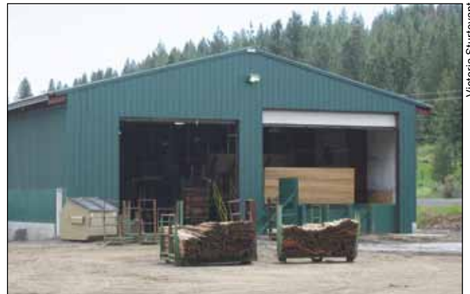
Figure 5-4—Bins of removed stickers outside the restacker where dry lumber is processed for shipping.
