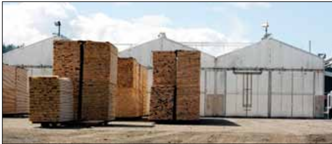
Figure 5-2—Green lumber waiting for kiln drying.
