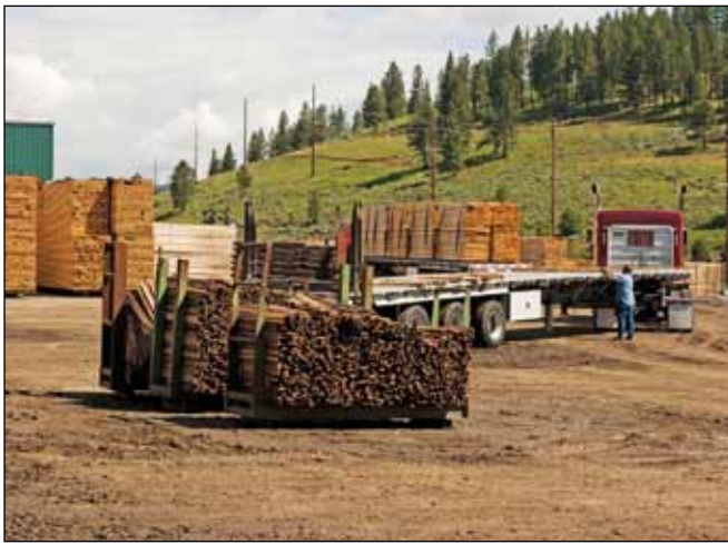
Figure 5-14—A truck carries twice the load when lumber is kiln dried.
