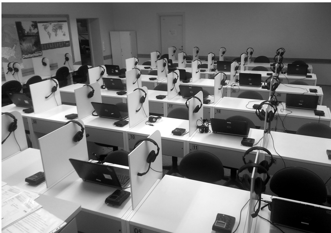
Figure 30: A classroom in pilot test configuration. The test was done on laptops recording through headsets. Though the screens and the seating patterns provide visual privacy, the acoustic environment has little in terms of isolation.
