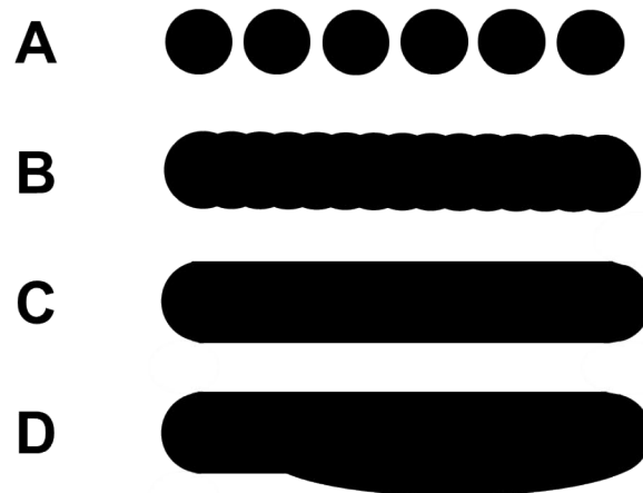
Fig. 9. Schematic illustration of drop spacing effect on boundary line edge of inkjet printed areas, showing drop spacing decreasing from A to D, with C presenting the cleanest edge.
