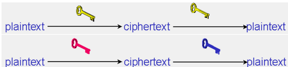
Figure 1.1: Top: Symmetric encryption using the same key, Bottom: Asymmetric encryption using different keys [Gar10].
