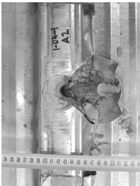
Fig. 16. Rib punch-through failure.
