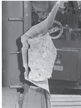
(b) Concrete failure surface, side view
