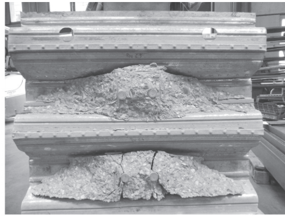
(a) Concrete failure surface, front view
