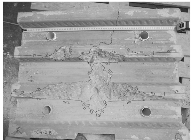
Fig. 18. Concrete pullout failure for the bottom rib and rib punch-through and stud failure for the top rib.
