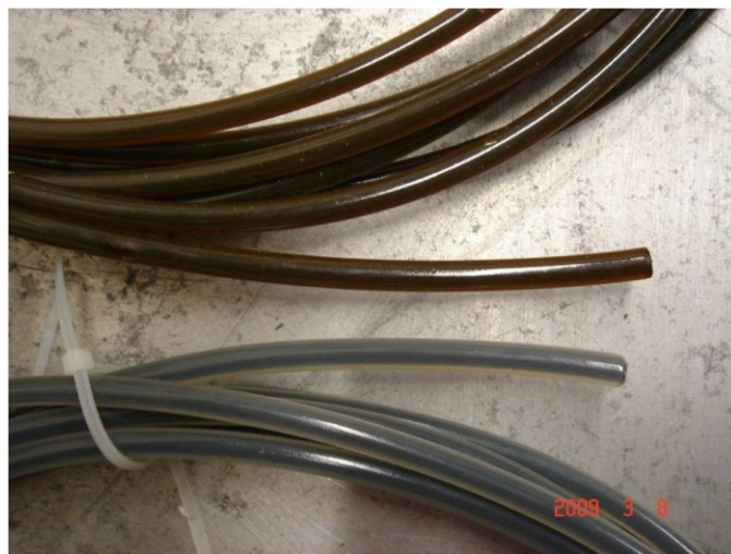
Figure 5: Comparison of aged (top) and un-aged model power cables.
