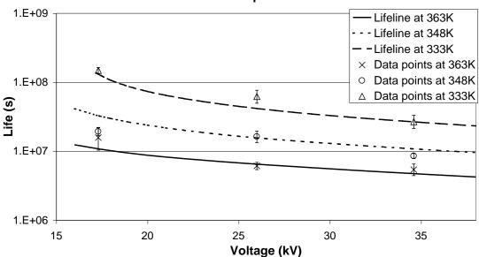
Application of thermoelectric ageing models to polymeric insulation in cable geometry
