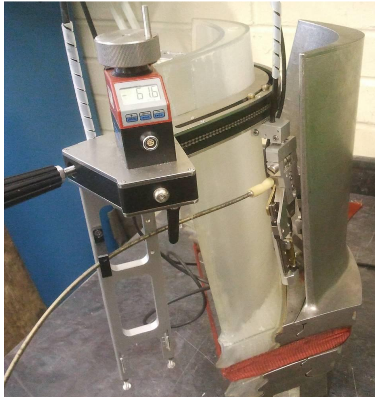
Figure 5-30 Bespoke scanning frame configured to scan the concave root from convex aerofoil
