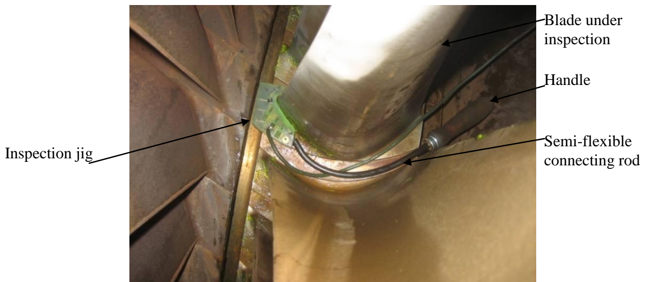
Figure 4-44 Finished leading edge inspection jig showing insertion from trailing edge to access the leading edge of blade root
