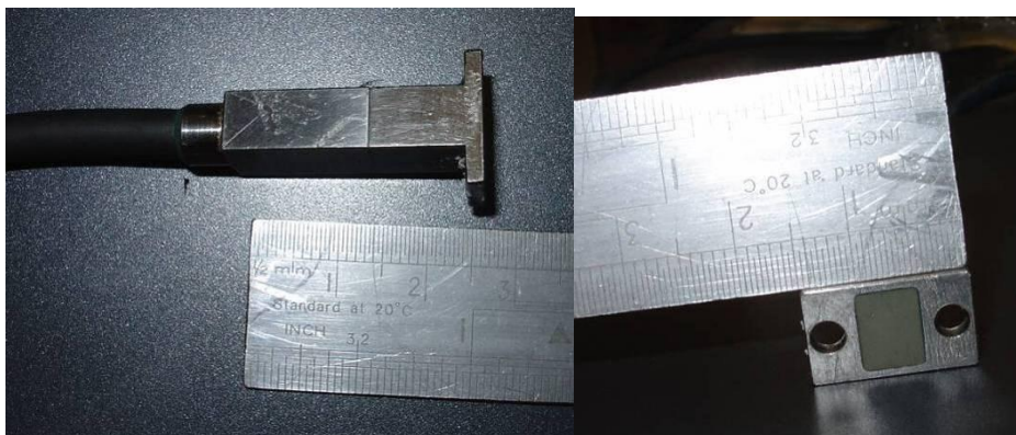
Figure B-1 Imasonic 6822 E101 - 10 MHz, 20 element phased array probe
