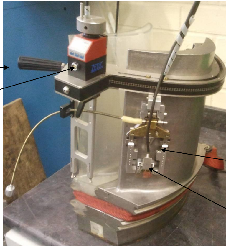
Figure 5-30 Bespoke scanning frame configured to scan the concave root from convex aerofoil
