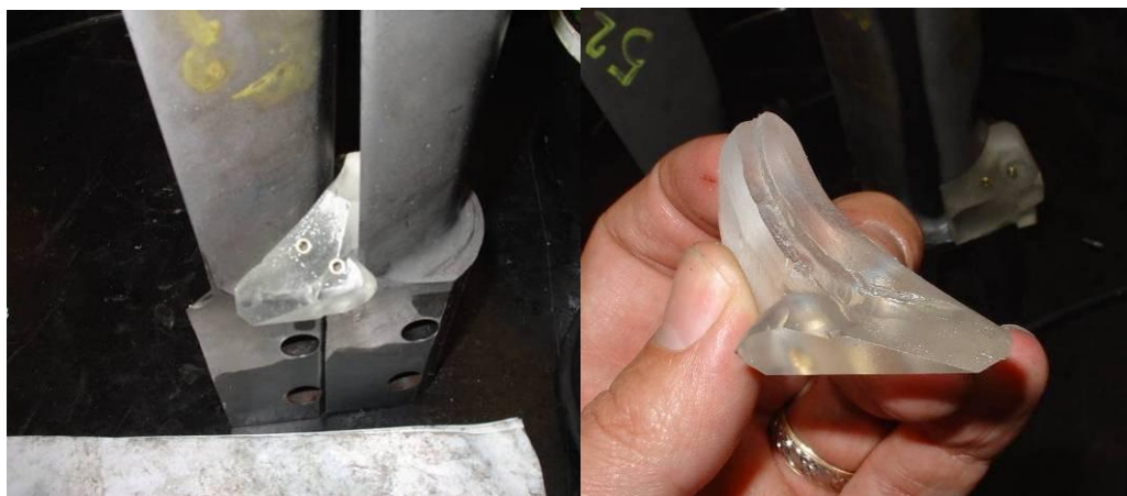
Figure 4-12 Zone 2b shear wave inspection jig
