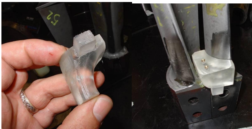
Figure 4-14 Zone 3 compression wave inspection jig
