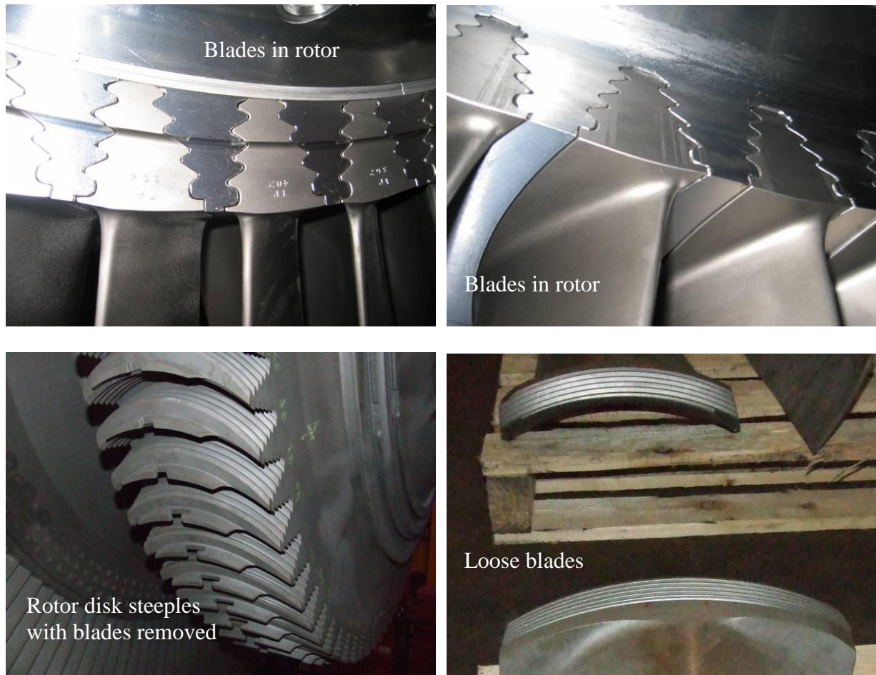
Figure 2-12 Curved axial entry fir tree roots
