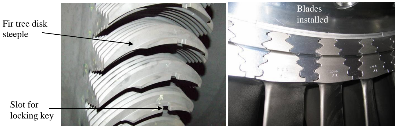
Figure 2-21 Disk head steep curved fir tree root slots
