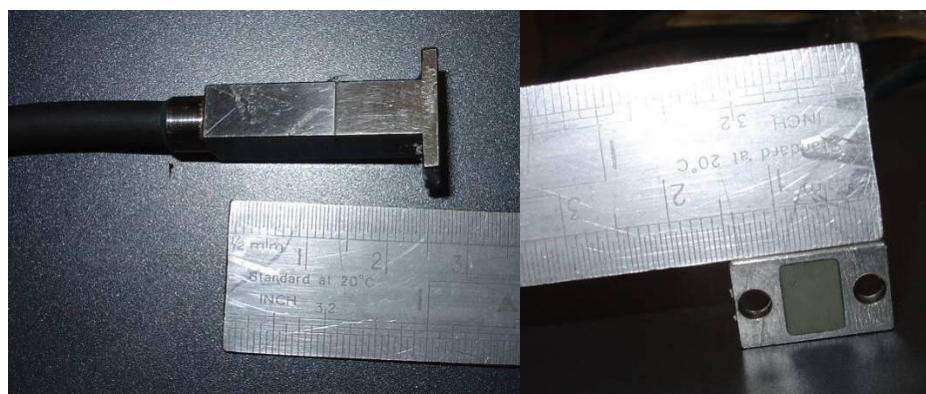
Figure 4-2 Imasonic 6822 E101 - 10 MHz, 20 element phased array probe
