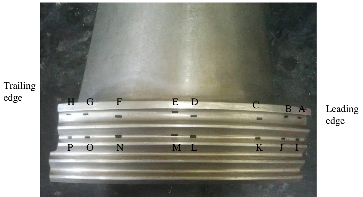
Figure 5-26 Reference sample S1 – convex root EDM notches
