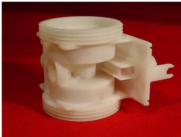
Figure 4-31 Example of a complex component manufactured by rapid prototyping
