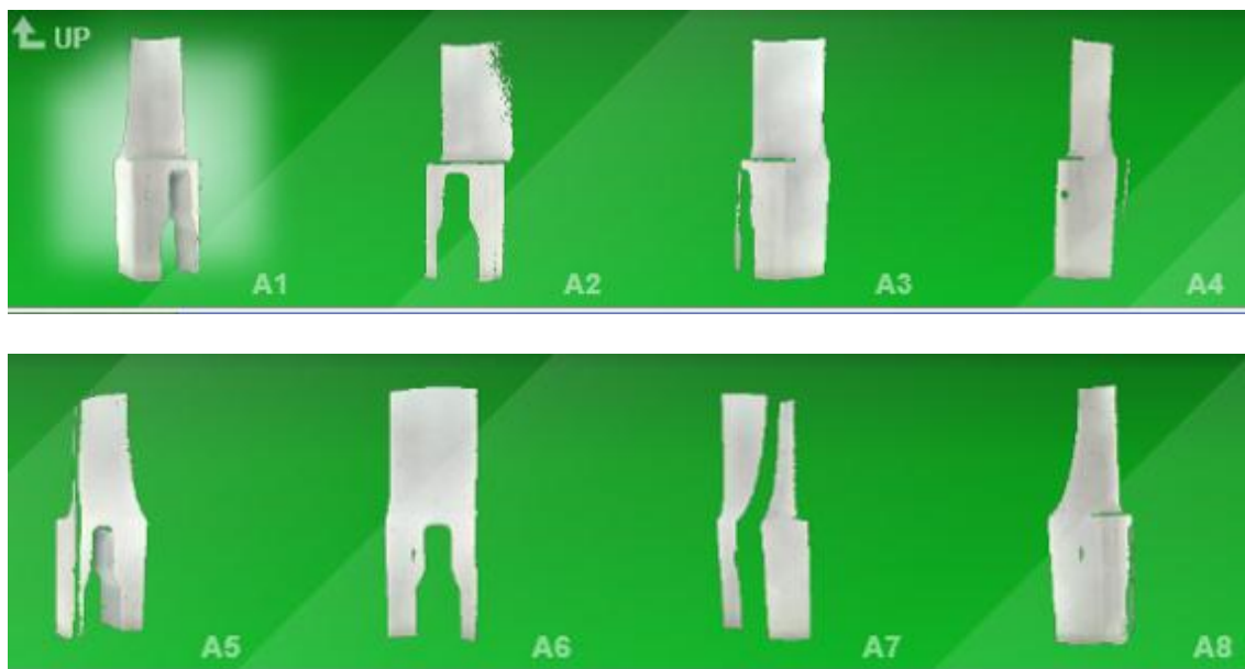
Figure 4-16 360° eight segment panoramic scan of stage 4 blade
