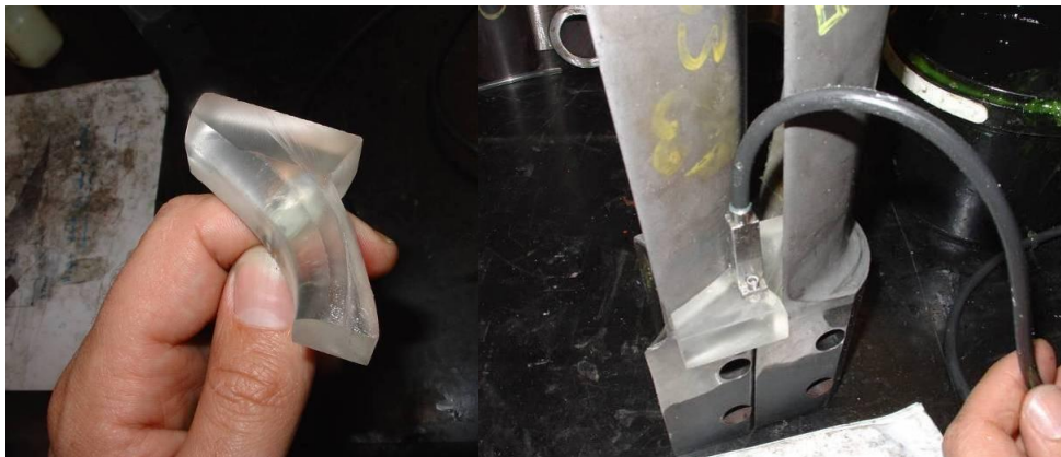
Figure 4-13 Zone 2a compression wave inspection jig
