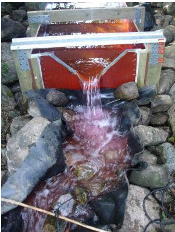
Figure 3-27. Dye trace and constructed flume at outlet of study pond.
