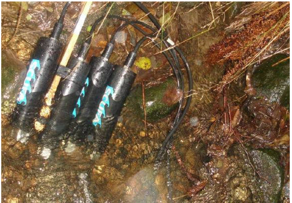
Figure 11-4. The installation of instruments for stream stability tests.
