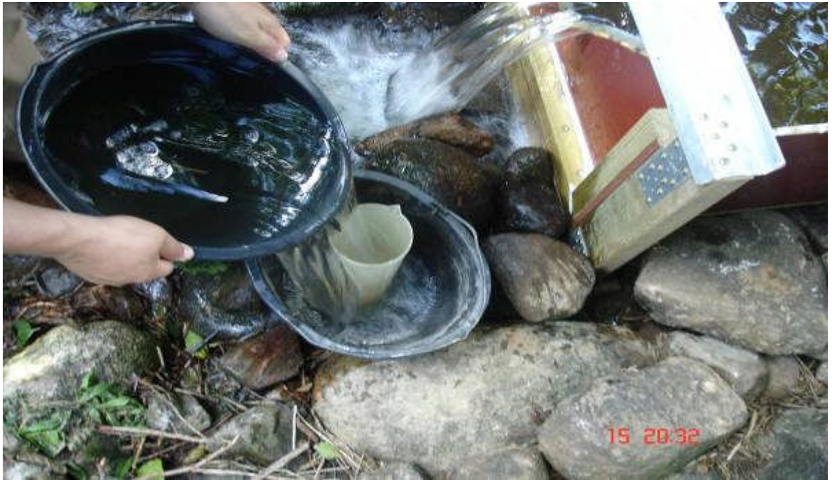
Figure 3-26. Volumetric (bucket) measurement.
