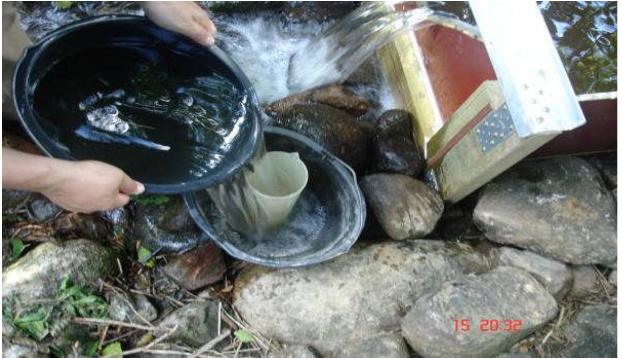
Figure 10-3. Volumetric (bucket) measurement.
