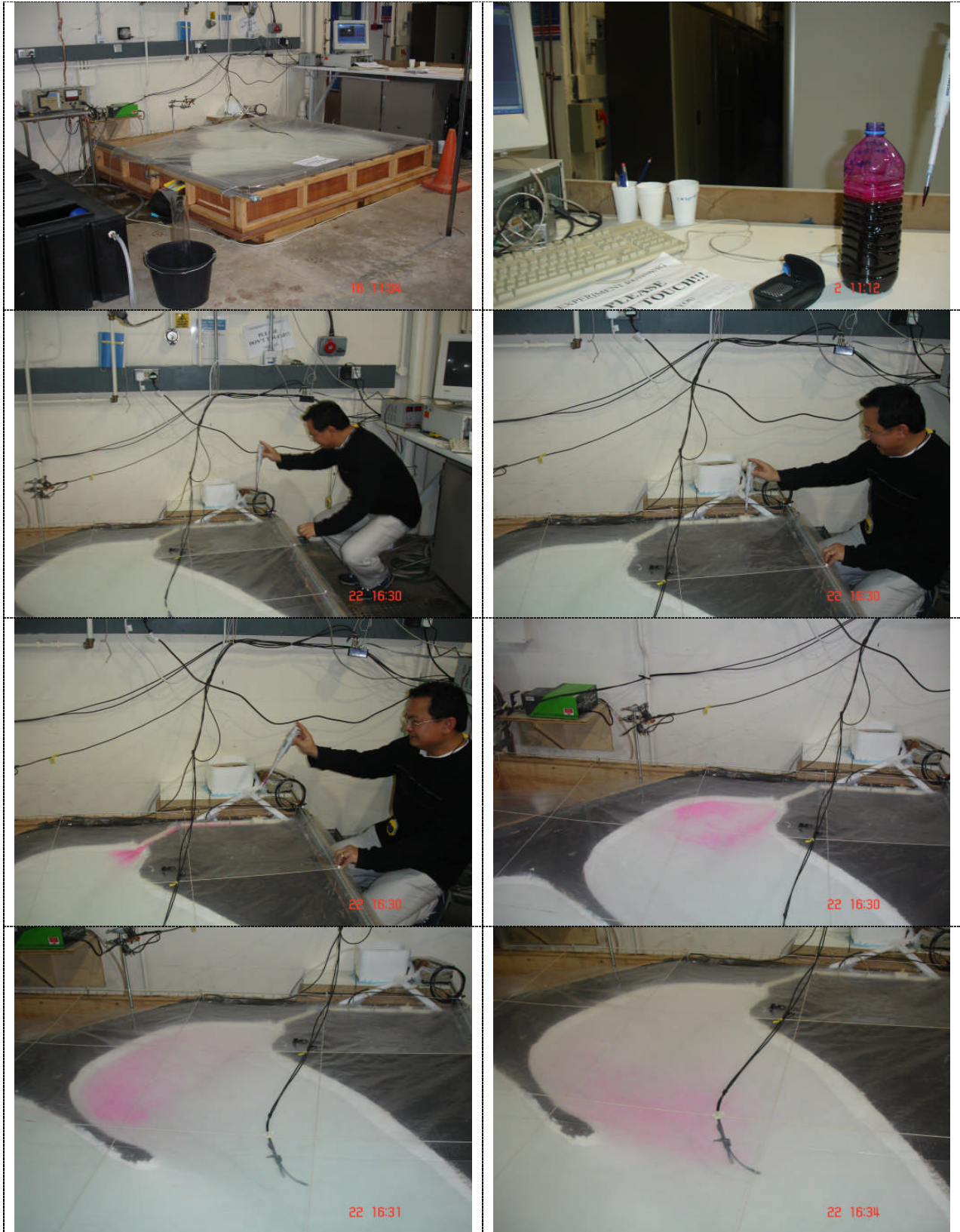
Figure 9-2. Pictures of Rhodamine dye test trace at Physical Scale Model Pond.
