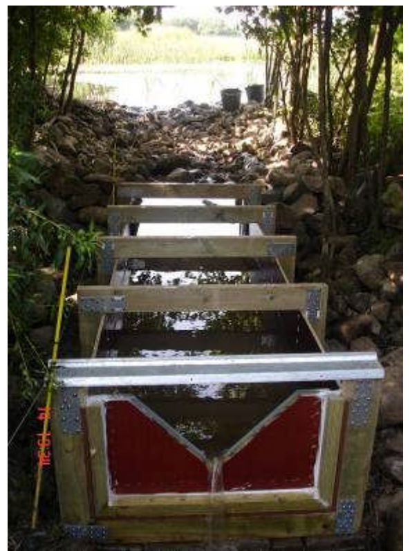
Figure 3-27. Dye trace and constructed flume at outlet of study pond.
