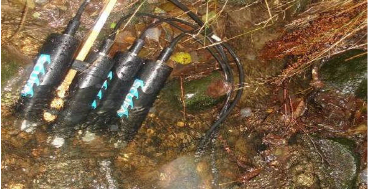
Figure 3-39. The installation of Scuba instruments for stream stability tested.
